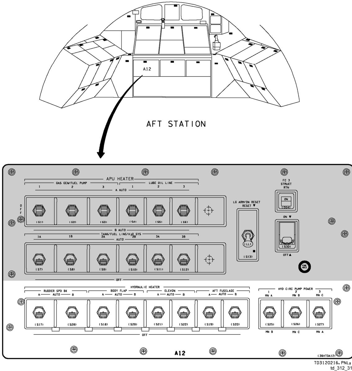
Figure 3-10. Panel A12 and its location
