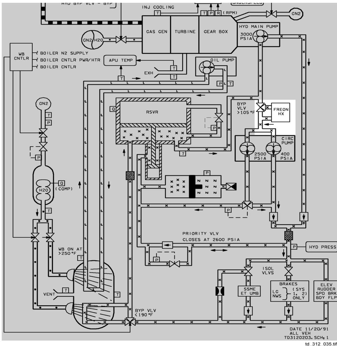
Figure 3-5. Hydraulic/freon heat exchanger
