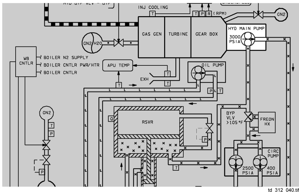
Figure 3-2. Hydraulic main pump
