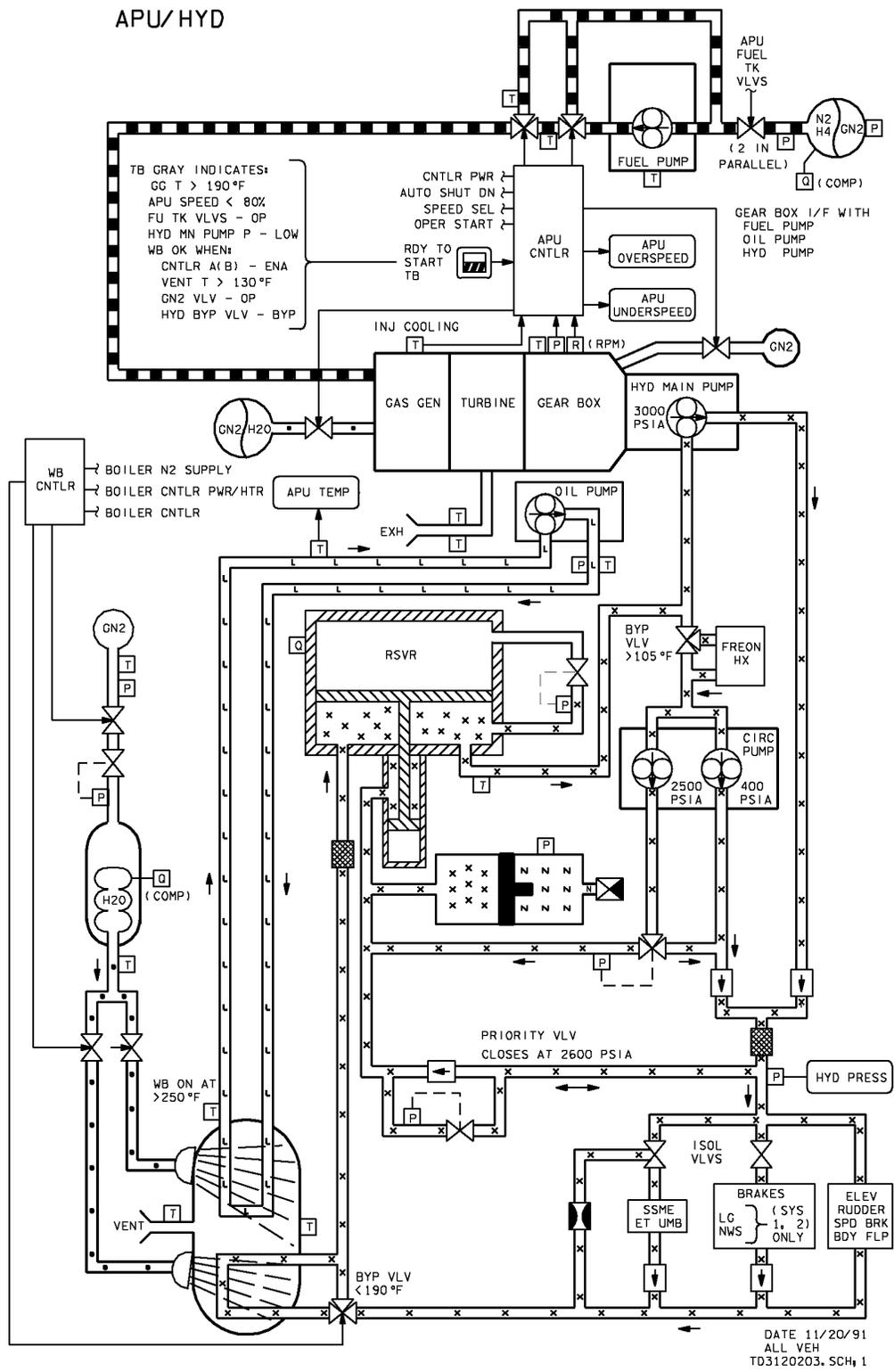
Figure 2-3. APU/HYD/WBS schematics
