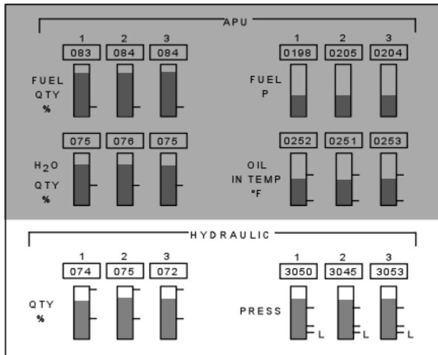
**Figure 3-13. HYD/APU Subsystem Status Display meters**
