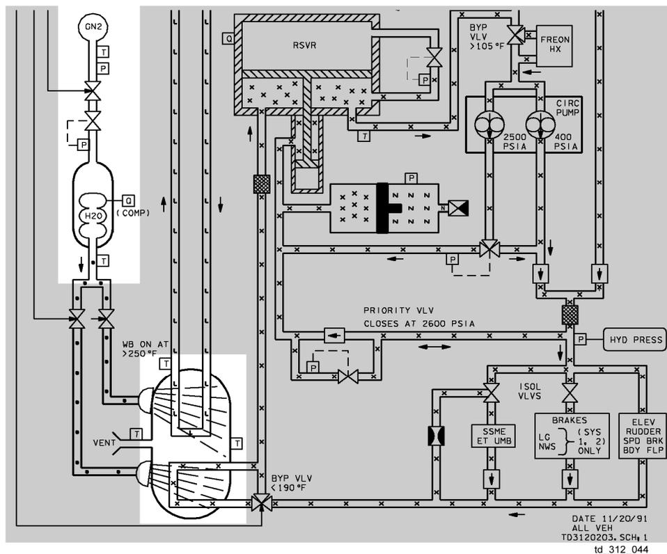
Figure 4-3. Water tank and boiler
