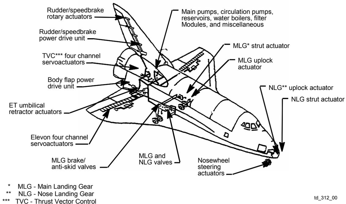
**Figure 3-1. Hydraulic system location**
