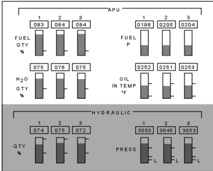
**Figure 2-17. HYD/APU Subsystem Status Display meters**
