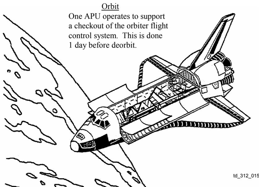
**Figure 5-4. APU/HYD/WSB system use on orbit**
