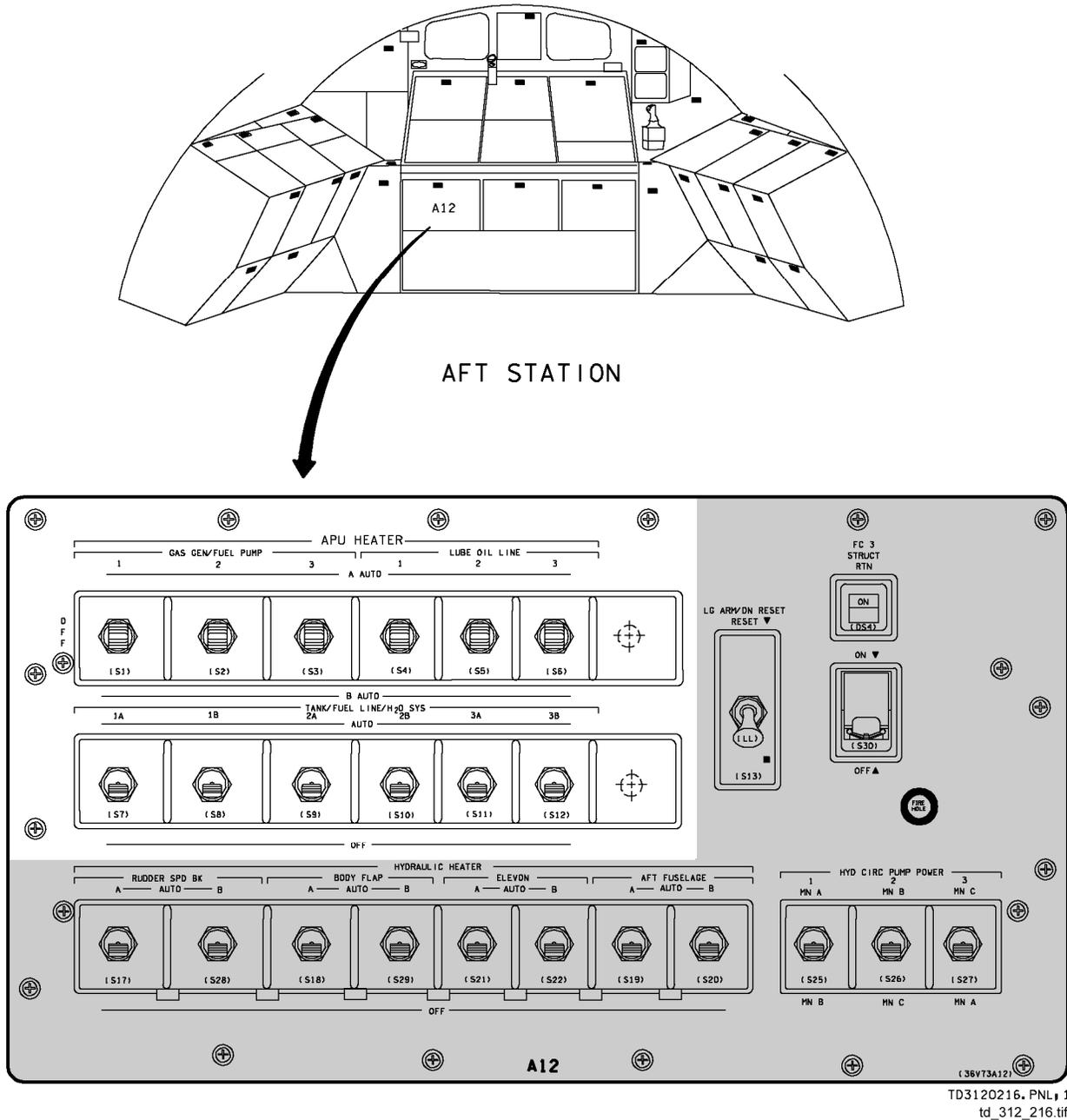
Figure 2-15. Panel A12 and its location
