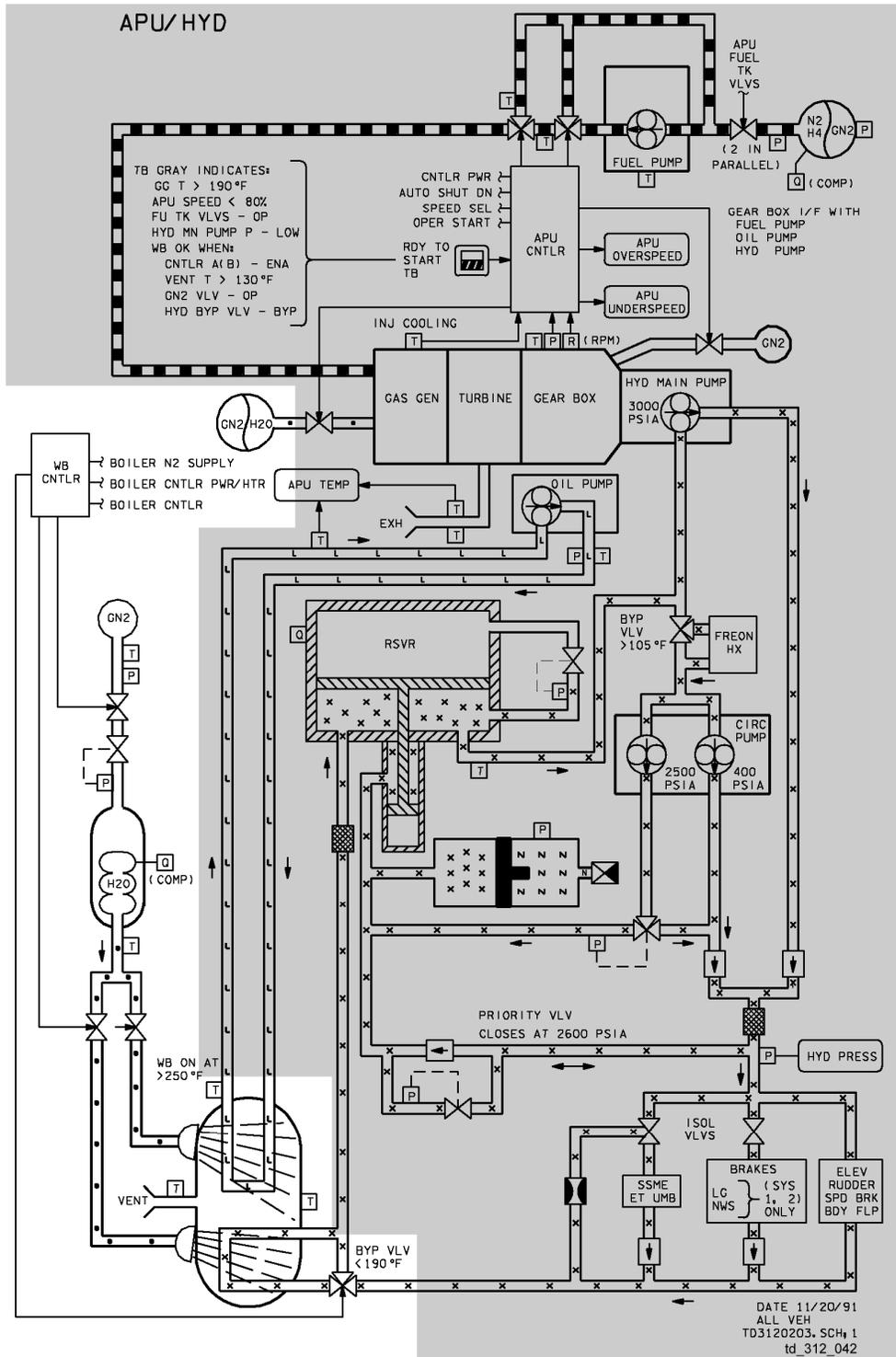
Figure 4-1. Water spray boiler system
